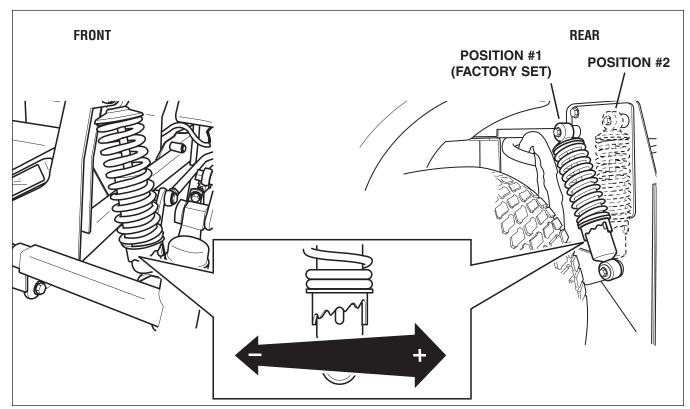
Figure 34. Suspension Adjustment
